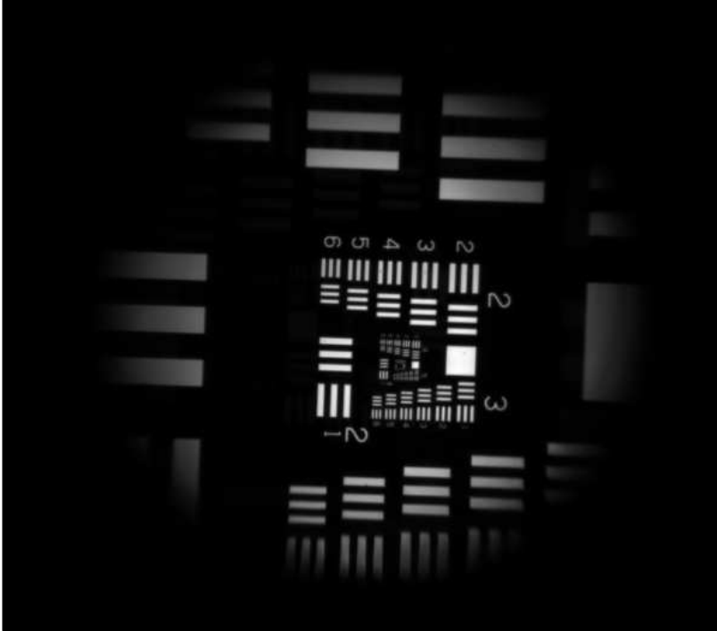
Figure 3: Air Force 1951 resolution test target image.
