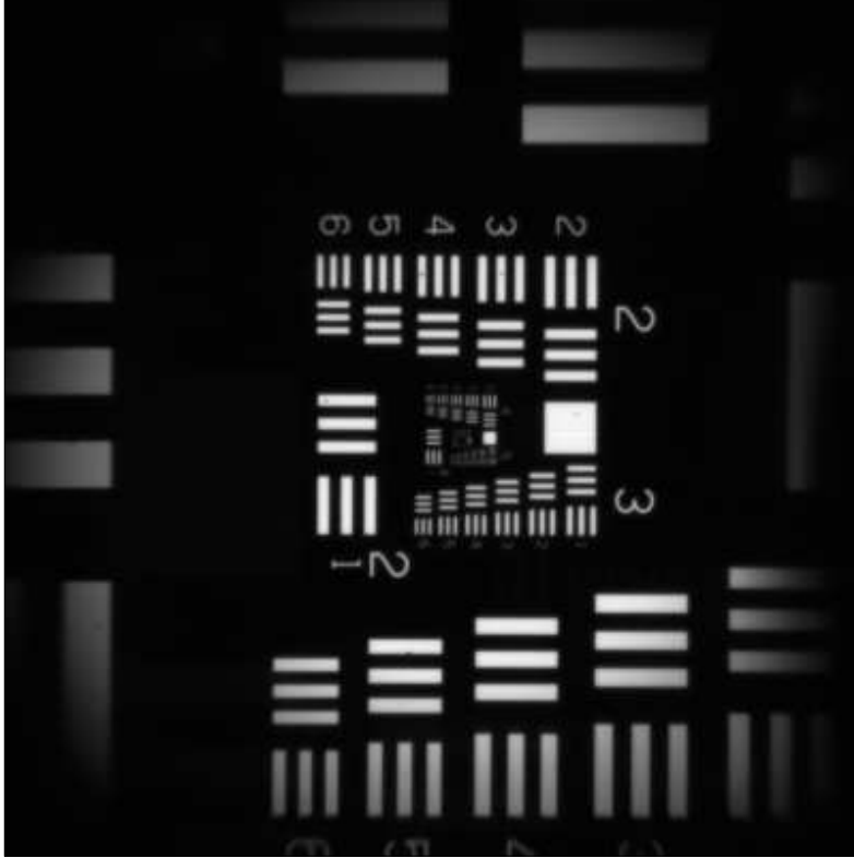
Figure 3: Sample Air Force target image in vacuum.
