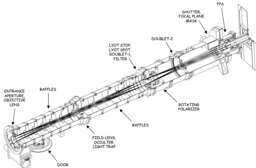
**Figure 1.** Layout of the COR1 instrument package.
